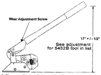
3. Measure distance between handle and bench. When properly adjusted, distance between inside edges of grip and bench is 17"+/- 1/2"for 5050B Tool
